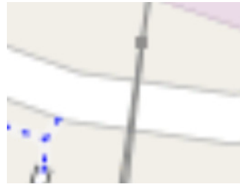
(b) Road crossing a power-line classified as a bridge.
